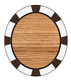
27mm thick, 35mm segmented edge length, 13deg mitre angle. 5mm spacing between segments.
